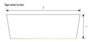
Size tolerance: Length +/-2% Width +/-0.5mm Thickness +/-0.2mm
